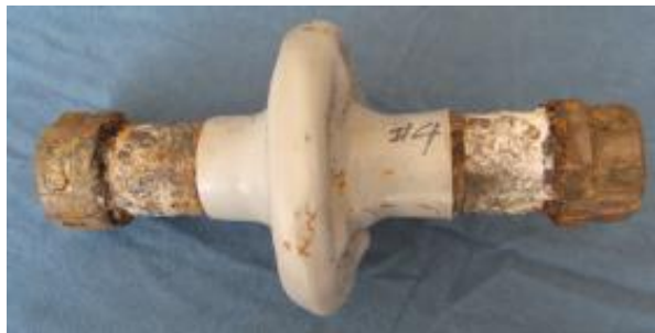
Fig.3E Flange #4 – After 3,000 Hr Salt Fog
