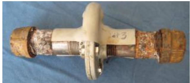
Fig.3D Flange #3-After 3,000 hr Sal Fog with a Cutout
