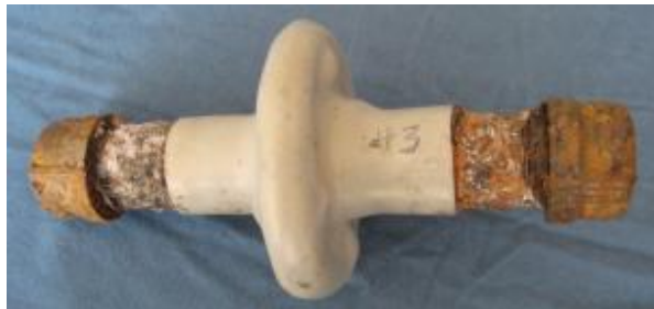
Fig.3C Flange #3 – After 3,000 Hr Salt Fog
