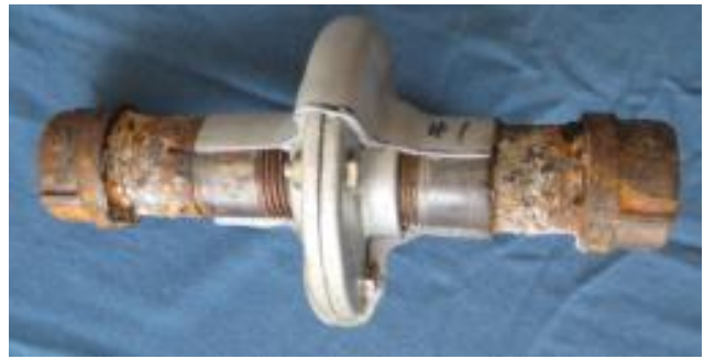
Fig.3B Flange #1-After 3,000 hr Sal Fog with a Cutout
