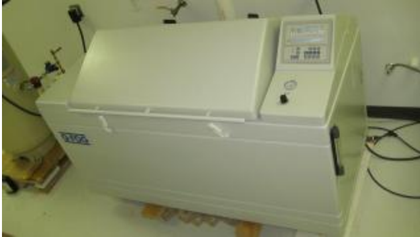
Figure 1 Q-fog Chamber for the Corrosion Resistance Testing, ASTM B117
