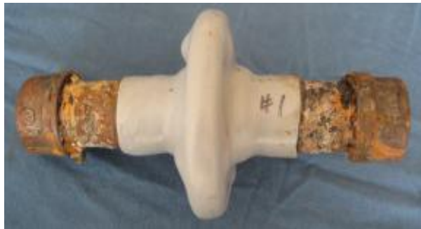
Fig.3A Flange #1 – After 3,000 Hr Salt Fog
